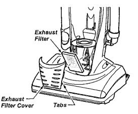
The exhaust filter removes dirt from recirculated air.
